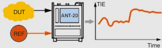
Fig. 32: Basic principle of wander measurement: Phase comparison between two clock signals
